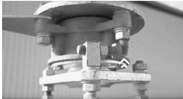
Fig. 19. Correct setting of the stop bolt
